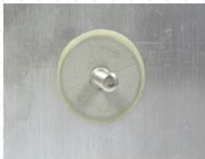
Step 7 Slowly turn part clockwise while pushing until it won't turn.
