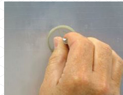
Step 6 Push part into the substrate to squeeze adhesive out from base.
