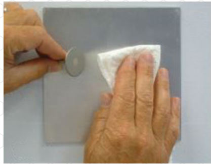
Step 1 Clean fastener and substrate with Scotchbrite (light scuff) and solvent.
